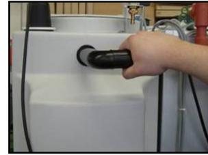
9. a) Remove the securing device of the submersible pump (cable tie on the tubes) in tanks 1 and 2 and suspend the pumps in the relevant tanks.
