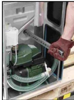
**Note: The service door on assembly 2 must never be placed under load during transport! To prevent damage to the UV lamp, there must be no mechanical load! Do not use tubing as carrying handles!**
